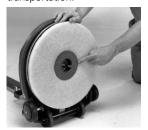
Permanent brush/pad holder mounted directly to motor. Eliminates transmission problems. Pad attaches easily to center mounting hub.
