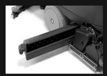
Counter-rotating cylindrical brushes deposit loose debris into hopper.
